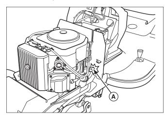
Figure 2. Manual Lift Adjustment Bolt A. Adjustment Bolt
